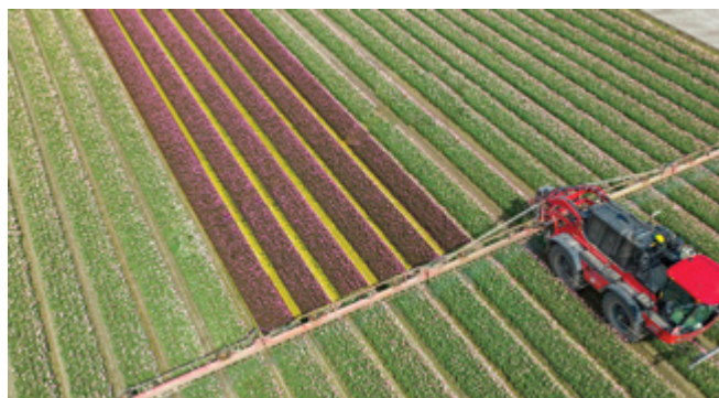
Variable Rate Application By Sections
